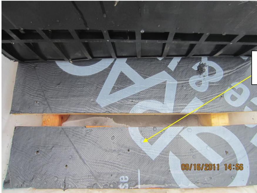
No ice or water infiltration observed after exposure
