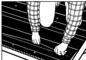
5. Install either felt (warm weather climates) or waterproof shingle underlayment (cold weather climates) over The Edge Vent being careful to avoid nailing into the roof deck slot. Using a chalk line, transfer the nail line (2 5/8" from drip edge) and slot location (5 3/4" to 7" from drip edge) to the top of the felt or waterproof shingle underlayment.
