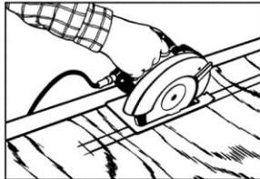
2. Cut slot with circular saw.
