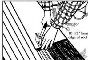
3. Making sure the slot is open from step #2, position The Edge Vent over slot. Make sure that the lower edge of the venting is aligned with the edge flashing. Start at end of roof so that end plug is flush with end. Locating tabs on underside of The Edge Vent may assist in positioning over slot. Use reinforced nail holes to pre-fasten vent in place.
