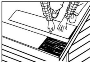
4. Use utility knife to cut final section to length. Integrated end plug of final section should be flush with end of roof. Pre-fasten final section.
