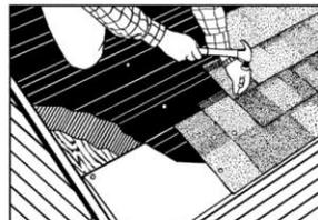
6. Install starter and first course shingles over felt/waterproof shingle underlayment-covered Edge Vent using shingle manufacturer guidelines for shingle overhang and nailing requirements. Nailing patterns may have to deviate from some shingle installation instructions to avoid nailing in slot location.
