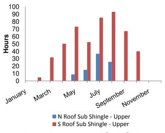
Figure 3. Time spent above 65.6°C (150°F) for upper shingles
