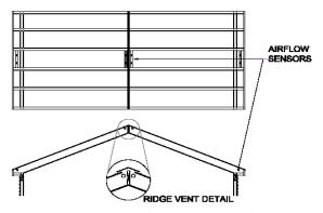
Figure 2. Illustration of sensor positions in test facility attic space
