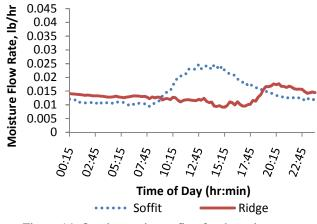
Figure 14. October moisture flux for the attic environment
