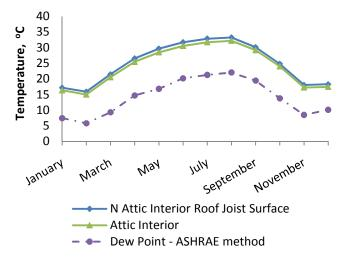
Figure 9. Monthly average temperature comparison for attic materials
