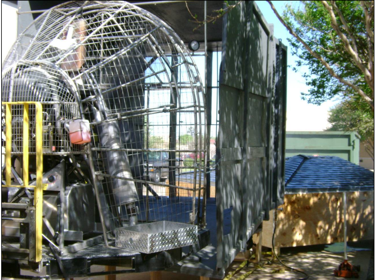
Photo No. 5: Wind generator and wind stream plenum (Specimen #1 in background)
