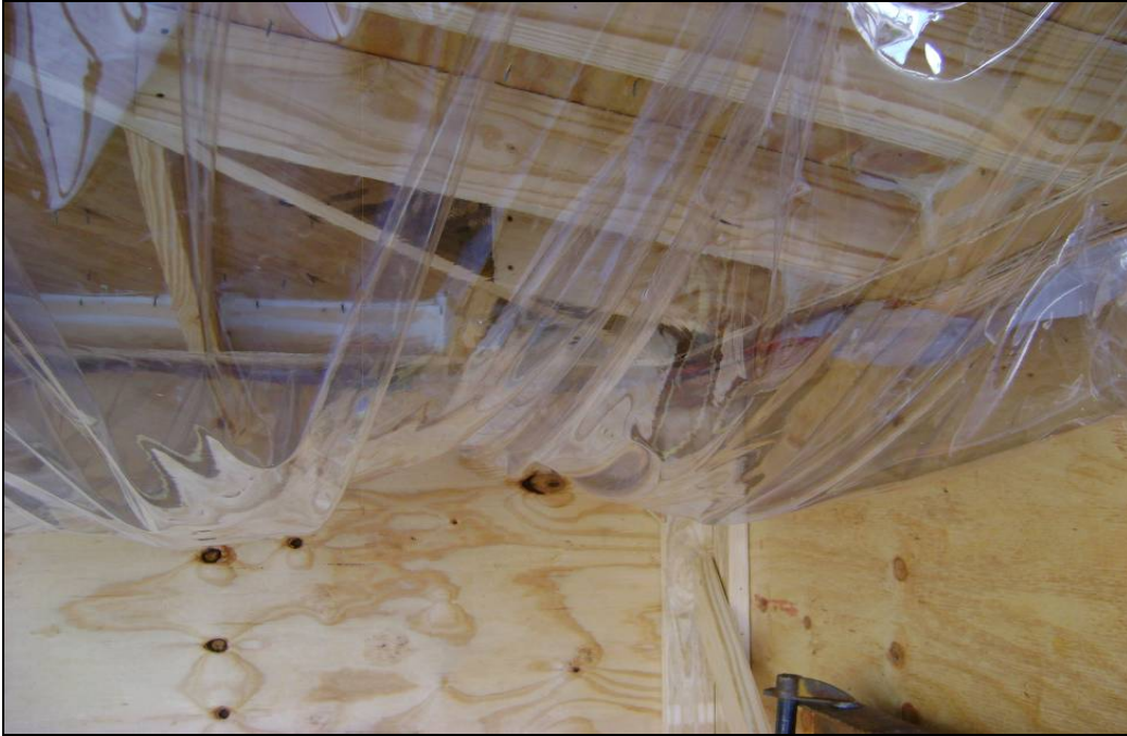
Photo No. 3: Water collection system under test deck at the conclusion of testing
