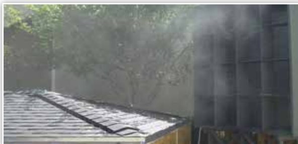
A wind generator with calibrated water spray system was used to subject Hip Ridge Vent to over 1,200 gallons of wind-driven rain at 35, 70, 90 and 110 MPH. The vent was tested on both a 3/12 and a 12/12 roof pitch. Hip Ridge Vent passed all the tests.
