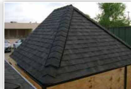
A wind generator with calibrated water spray system was used to subject Hip Ridge Vent to over 1,200 gallons of wind-driven rain at 35, 70, 90 and 110 MPH. The vent was tested on both a 3/12 and a 12/12 roof pitch. Hip Ridge Vent passed all the tests.
