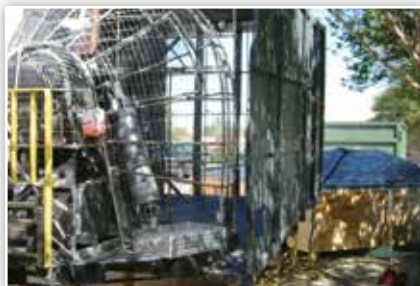
A wind generator with calibrated water spray system was used to subject Hip Ridge Vent to over 1,200 gallons of wind-driven rain at 35, 70, 90 and 110 MPH. The vent was tested on both a 3/12 and a 12/12 roof pitch. Hip Ridge Vent passed all the tests.
