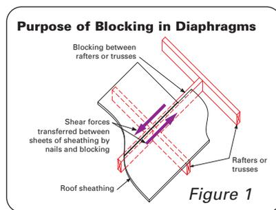
In **unblocked diaphragms**, this shear force transfer can only occur at the main framing members (rafters or trusses.) This is why the allowable design loads in unblocked diaphragms are so much lower than those possible with blocked diaphragms.
