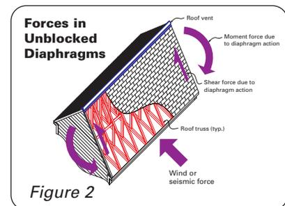
In unblocked diaphragms, the bending moments and shear are both resisted by the sheathing.
