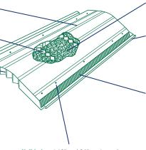
Nail holes at 16" and 24" center make it easy to locate and nail through studs.
