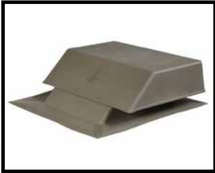
SLP150 Slant Back Plastic 24" x 24" flashing NFA: 150 sq. in./pc. 13" square opening
