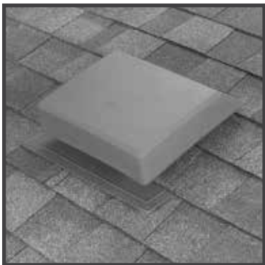
SLP61 Slant Back Plastic 16.5" x 19.5" flashing NFA: 61 sq. in./pc. 9" square opening CSA approved
