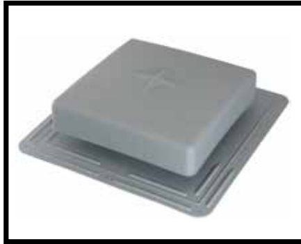
RVP61 Square Plastic 17" x 18" flashing NFA: 61 sq. in./pc. 9" square opening
