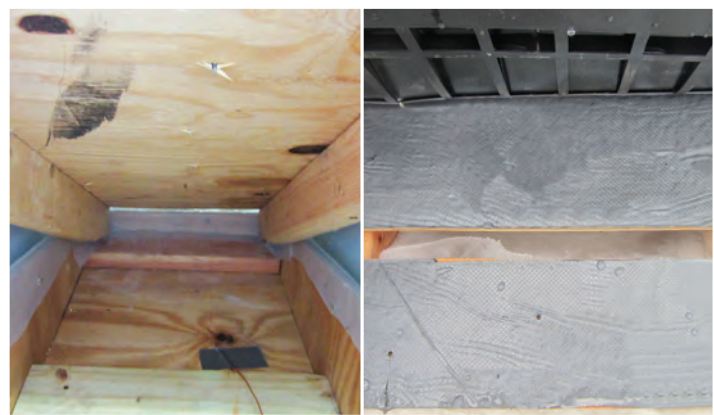
The deck under The Edge Vent and the attic itself remained dry throughout the 30-day ice dam test.
