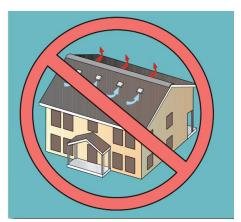
One of the most potentially troublesome attic ventilation mistakes is having <u>two</u> <u>different types of exhaust vents</u> on your house – for example, mixing a ridge vent with a powered fan, a roof louver, a gable louver or a wind turbine. Technically, this mistake is called short-circuiting the attic ventilation system. (*See illustration on the left.*)
