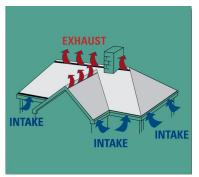
Research has shown that the best way to ventilate an attic is with a **balanced system** of intake vents low at the roof's edge or in the soffit/eaves along with exhaust vents high on the roof at or near the ridge. This allows cool, dry intake air at the roof's edge to flush out any warm, moist air through the exhaust vents.
