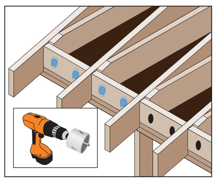
Mini Louvers are used to seal existing rafter/bird block vent holes to maximize airflow while protecting against rodent and insect invasion.
