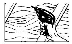
**3. CUTTING THE HOLE:** Draw a circle 14½" in diameter using the guidehole as the center. A template is provided on the back of the carton for drawing the circle.
