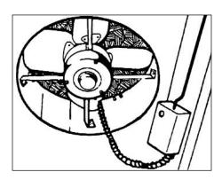
WIRING THE THERMOSTAT: Wire the thermostat as shown below. Attach your ground wire to the thermostat box.
