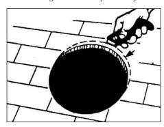
**5. SECURING THE BASE:** Make sure the base flange parallels the ridgeline of the roof. The embossed arrow and word UP should be pointing toward the ridgeline. Slip the upper half of the flange under the shingles.
