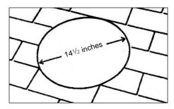
**4. CUTTING THE HOLE IN THE ROOF:** Using a sabre saw, cut and remove all roof shingles (and deck) inside the 14½"-diameter circle. Next, cut an extra 1" off the top half of the hole (shingles only) to allow room for placing and positioning the flange. Do not cut through any rafters. Cutting a rafter may cause your roof to sag.
