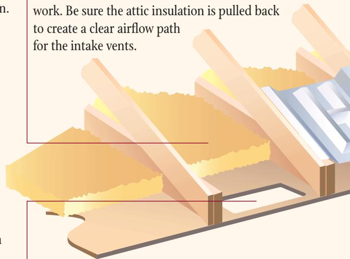
❑ **Go far out on the rafter tail.** Position intake vents as far out on the rafter tail as possible. Doing this will provide an optimum airflow path from intake to exhaust. Furthermore, it will help prevent the intake vent from being blocked by the attic insulation.
